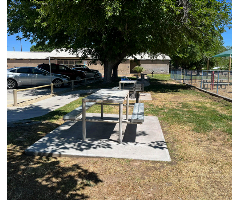
Add sidewalks and accessible ramps at three locations to provide ADA access. Remove old picnic table and concrete pads or replace with ADA accessible table and connecting sidewalks.
