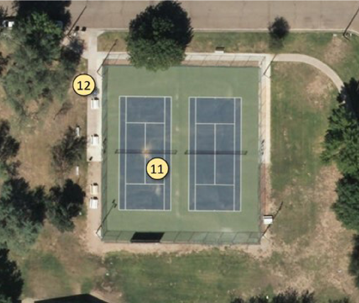
ITEM 11 – Minor court repair at net and seal cracks in court. ITEM 12 – Replace chain link fence.
