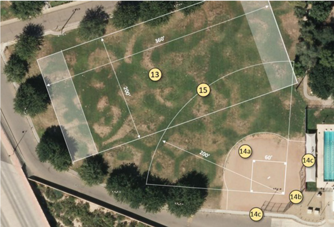
ITEM 13 – Repair field suitable for football and/or soccer program. ITEM 14a – Replace sand infield with regulation infield mix. ITEM 14b – Remove and replace chain link backstop fence. ITEM 14c – Add dugout fencing and benches. ITEM 15 – Provide temporary outfield fence for baseball.
